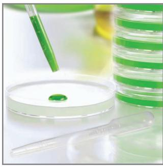
Globe Scientific is pleased to introduce these disposable wide bore transfer pipets. These pipets feature a wide tip opening designed specifically for the transfer of viscous liquids and small particulates. They are useful in the biofuel, petroleum, water treatment, food/beverage and pathology industries. The pipets are manufactured from low-density polyethylene (LDPE) and are packaged in convenient dispenser boxes; 500 pipets/box, 10 boxes/case.
